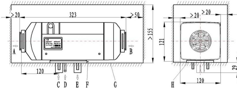
A-Inlet of heating air    B-Outlet of heated air    C-Inlet of combustion air
